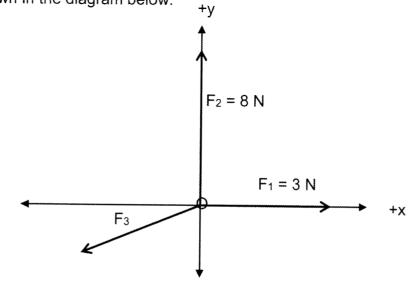
$F_1$  is a 3 N force, acting at 90<sup>o</sup> and  $F_2$  is a 8N force acting at at 0<sup>o</sup>.  $F_3$  has an x-component of -4 N and a y-component of -3 N.
