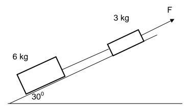
The coefficient of kinetic friction for the 3 kg object and the 6 kg object is 0.1 and 0.2 respectively.
