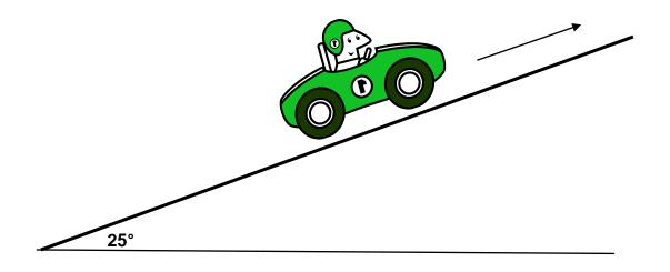
A car with a mass of 1 400 kg is accelerated up a hill while experiencing a net force of 7400 N. The hill makes an angle of  $25^{\circ}$  with the horizontal and the coefficient of dynamic friction is equal to 0, 23.
