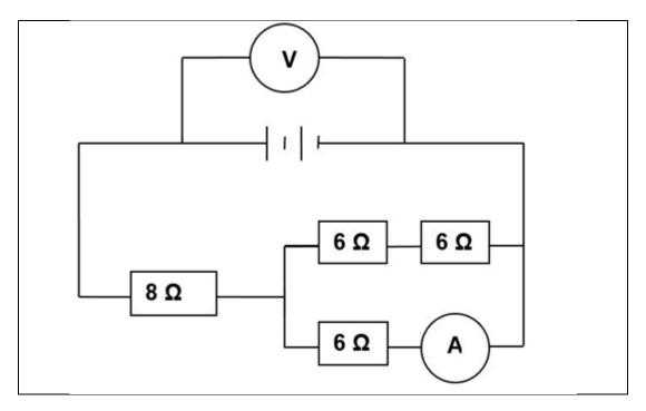
The power of the 8  $\Omega$  resistor is 0,5 W.
